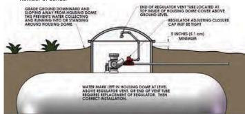
Figure 5: Underground Installation
