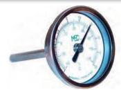
Designed for use in LP-Gas or  $\mathrm{NH_3}$  storage tanks, nurse tanks, bobtails and transports. These stainless steel, dust and water proof thermometers feature a 1/2" MNPT connection with a temperature range from  $-40^{\circ}$  to  $+120^{\circ}$  Fahrenheit. Accuracy +/-1 percent full range.
