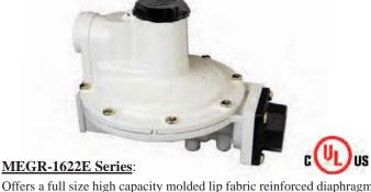
Offers a full size high capacity molded lip fabric reinforced diaphragm, stainless steel internal components, fluorocarbon (FKM) seat discs, precision machined aluminum orifices, and an adjustment range from 1.0-2.2 PSI (factory set @ 2 PSI) providing superior downstream regulation and maximum corrosion resistance against weather or contaminated gas.
